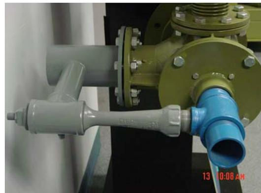
Fig. 14. Hauck Patented External FGR System
