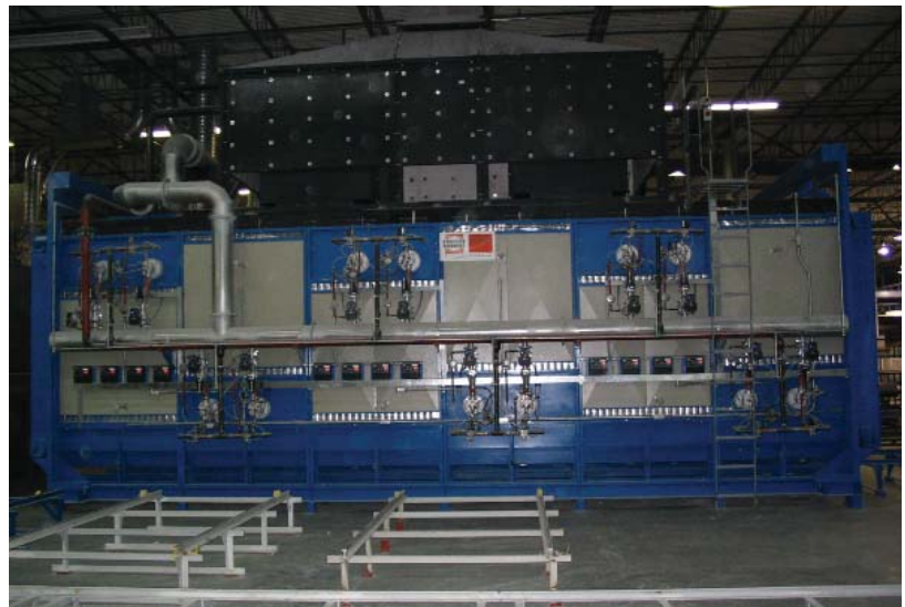
The kiln is equipped with Kromschröder high-performance burners and control components.
